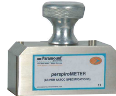
Calibrated Dead Weight (Made of Stainless Steel)
