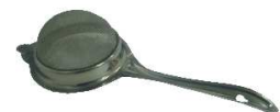
Filter Unit (For taking out the S.S. Balls from the Beakers after testing.)
